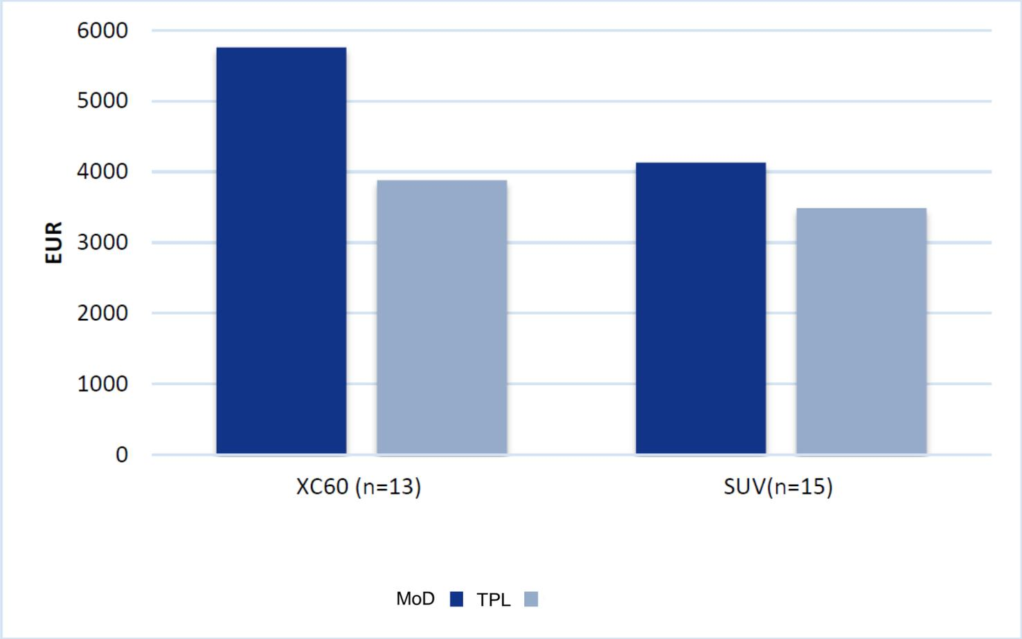
MoD and TPL repair costs of Volvo XC60 are higher because of higher material costs due small overlap
